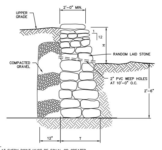
1. "T" AT EVERY POINT MUST BE EQUAL OR GREATER THAN H/2. 2. THE FIELDSTONE WALLS DESIGN SHOULD ONLY BE USED FOR VERTICAL GRADE SEPARATIONS OF 6 FEET OR LESS ON SITE.
