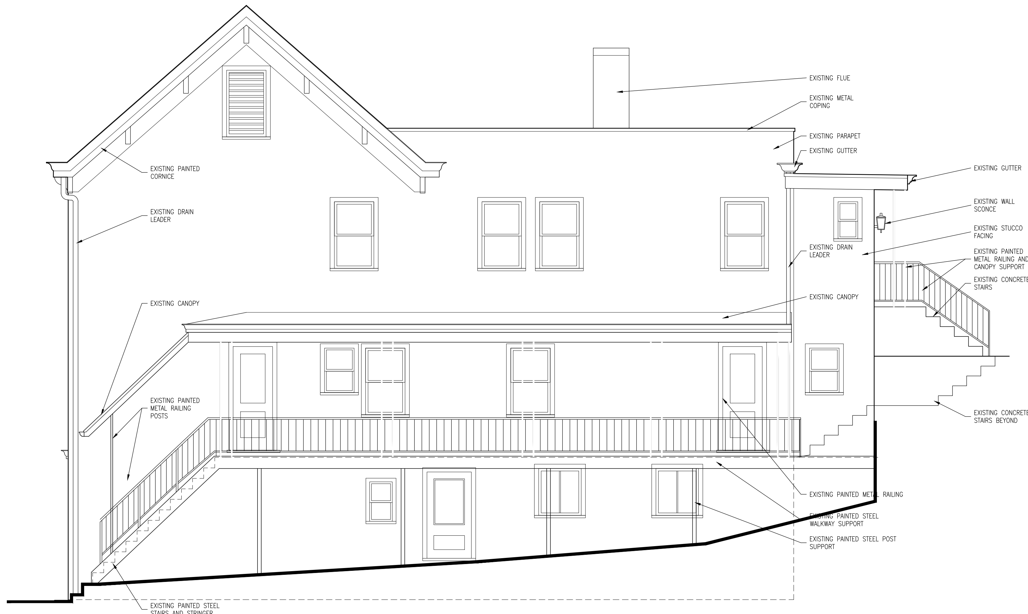
2 EXISTING SOUTH ELEVATION 1/4"=1'-0"
