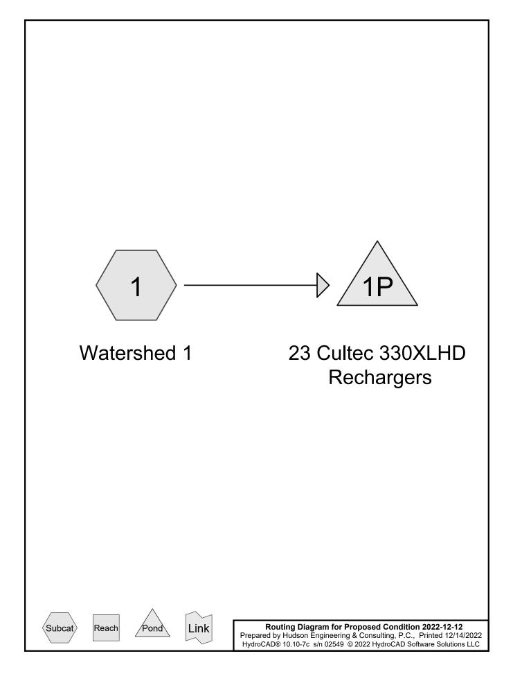
Proposed Condition 2022-12-12 Prepared by Hudson Engineering & Consulting, P.C. HydroCAD® 10.10-7c s/n 02549 © 2022 HydroCAD Software Solutions LLC
