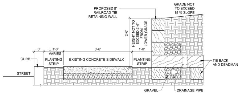
**SECTION - PROPOSED RETAINING WALL**
