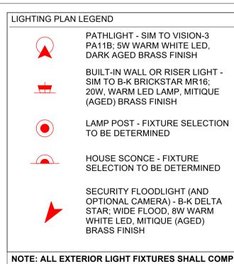
NOTE: ALL EXTERIOR LIGHT FIXTURES SHALL COMPLY WITH VILLAGE EXTERIOR LIGHTING CODE REQUIREMENTS (300-41), INCLUDING THE USE OF FULL **CUTOFF STYLE FIXTURES WITH LIGHT LEVELS WITHIN** THE LIMITS SET BY THE CODE.
