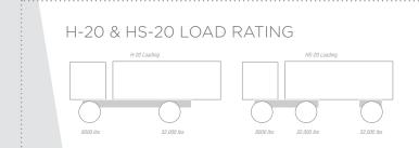
Similar to top of deck stresses per AASHTO H-20 loading conditions (32,000 lbs/14,500 kg), Unilock pavers can support 3-4 axle vehicles. This would include delivery, fire and semi-truck and trailer traffic in light-duty roadway applications.
