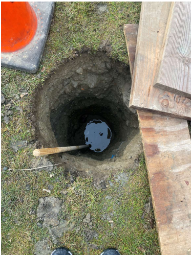
Percolation test initial conditions (fully saturated)
