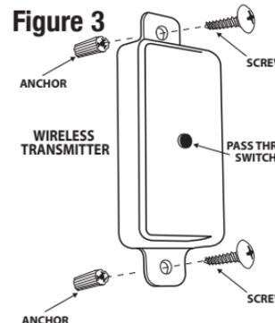
The Outdoor Wireless Transmitter must be installed at least 54 inches above the threshold of the door. The battery is already installed in the transmitter. Mount the transmitter with the 2 remaining larger supplied screws.
