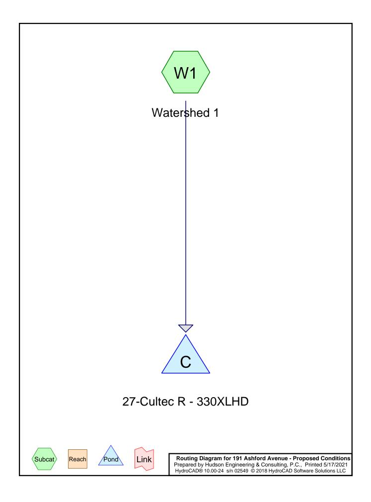
Time span=0.00-60.00 hrs, dt=0.01 hrs, 6001 points Runoff by SCS TR-20 method, UH=SCS, Weighted-CN Reach routing by Stor-Ind+Trans method - Pond routing by Stor-Ind method
