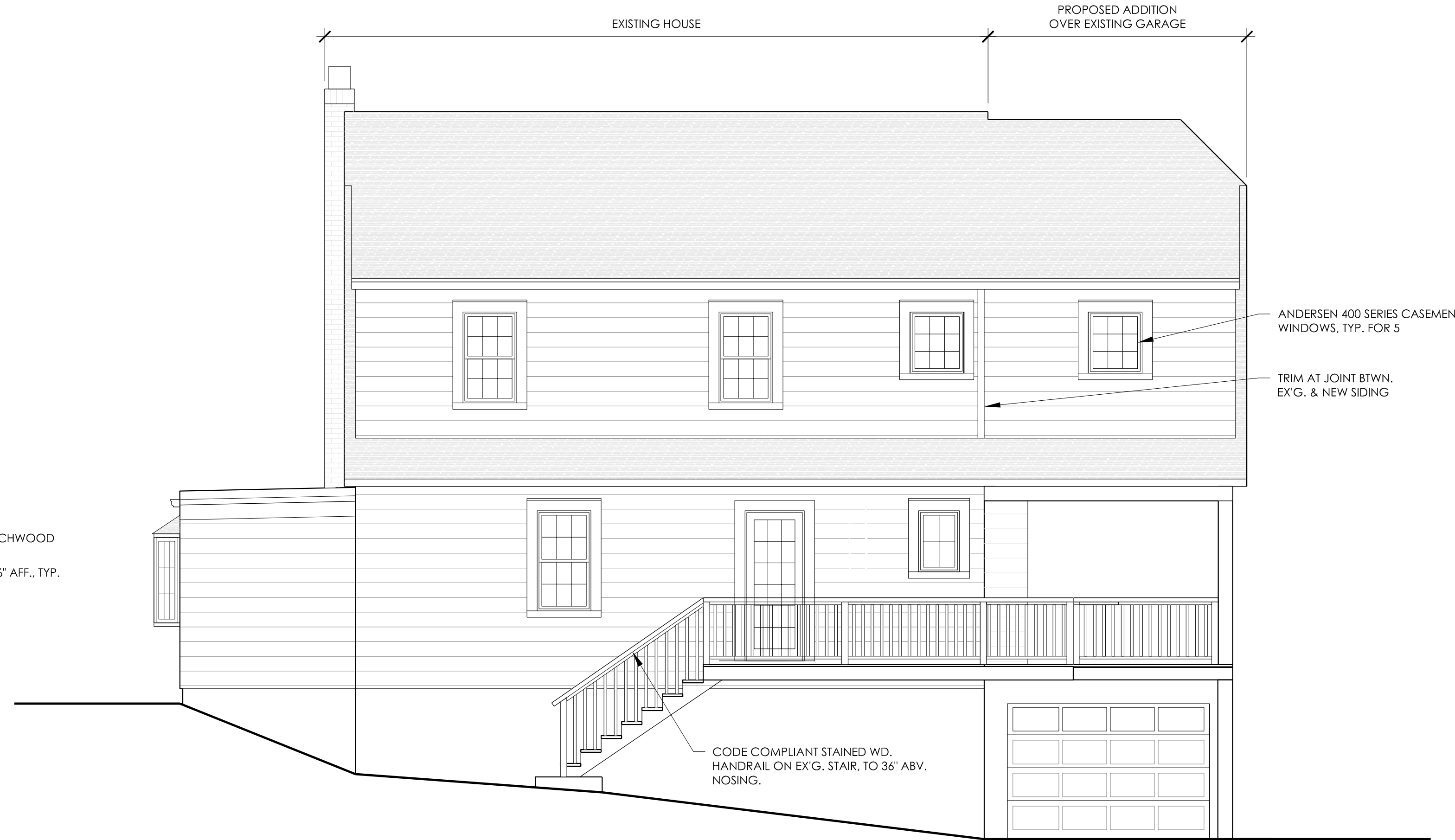
2 EAST ELEVATION SCALE: 1/4" = 1'-0"
