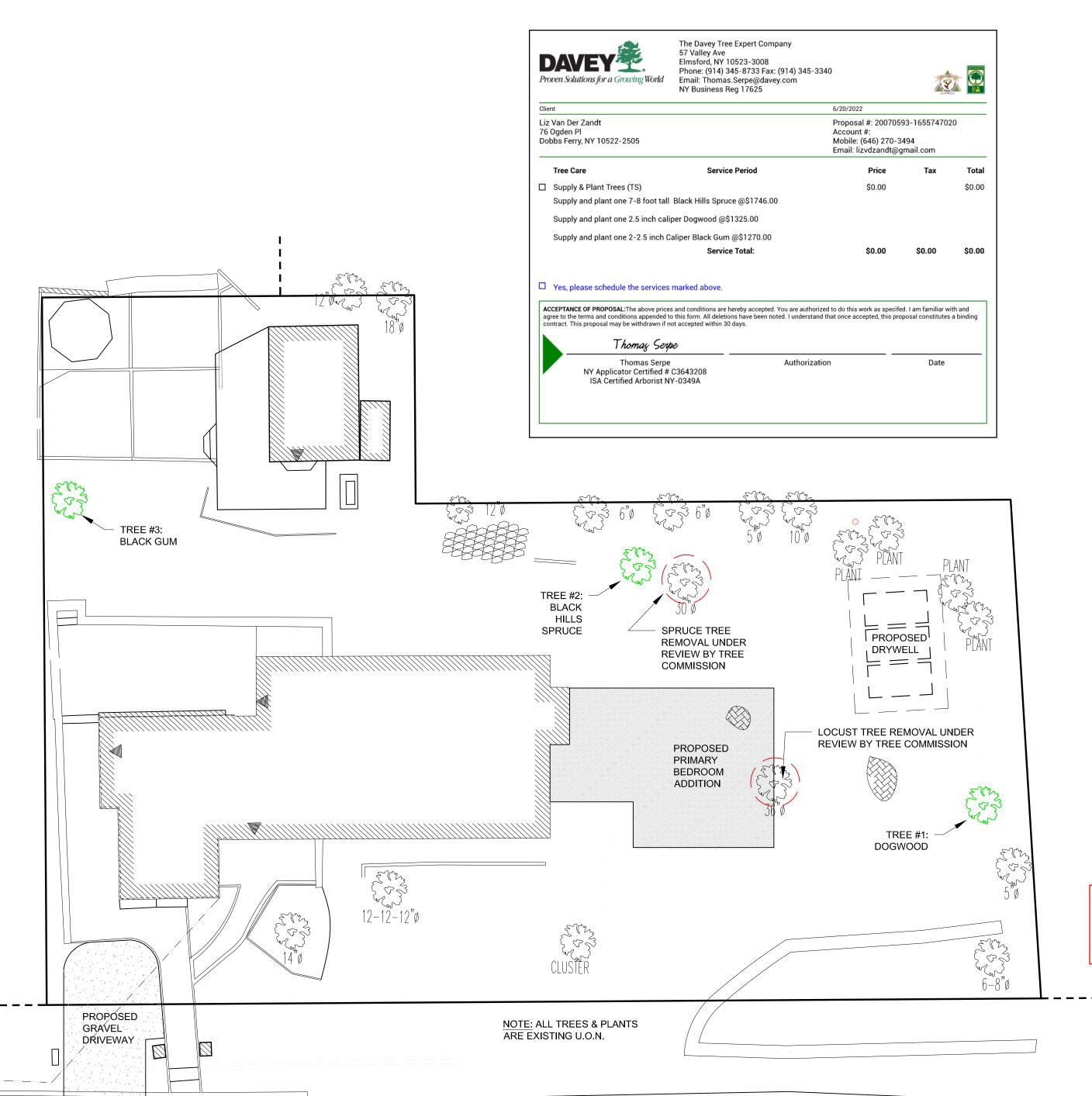
NOTE: PROPOSED TREE PLANTING LOCATIONS SHOWN PRESUME THE APPROVAL AND CONSTRUCTION OF THE PROPOSED ADDITION AND DRYWELL. THE TREE LOCATIONS MAY NEED TO BE REVISED BASED ON SITE CONDITIONS.
