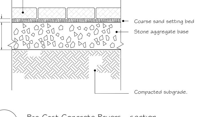
Pre-Cast Concrete Pavers - section Scale - |" - |.0'
