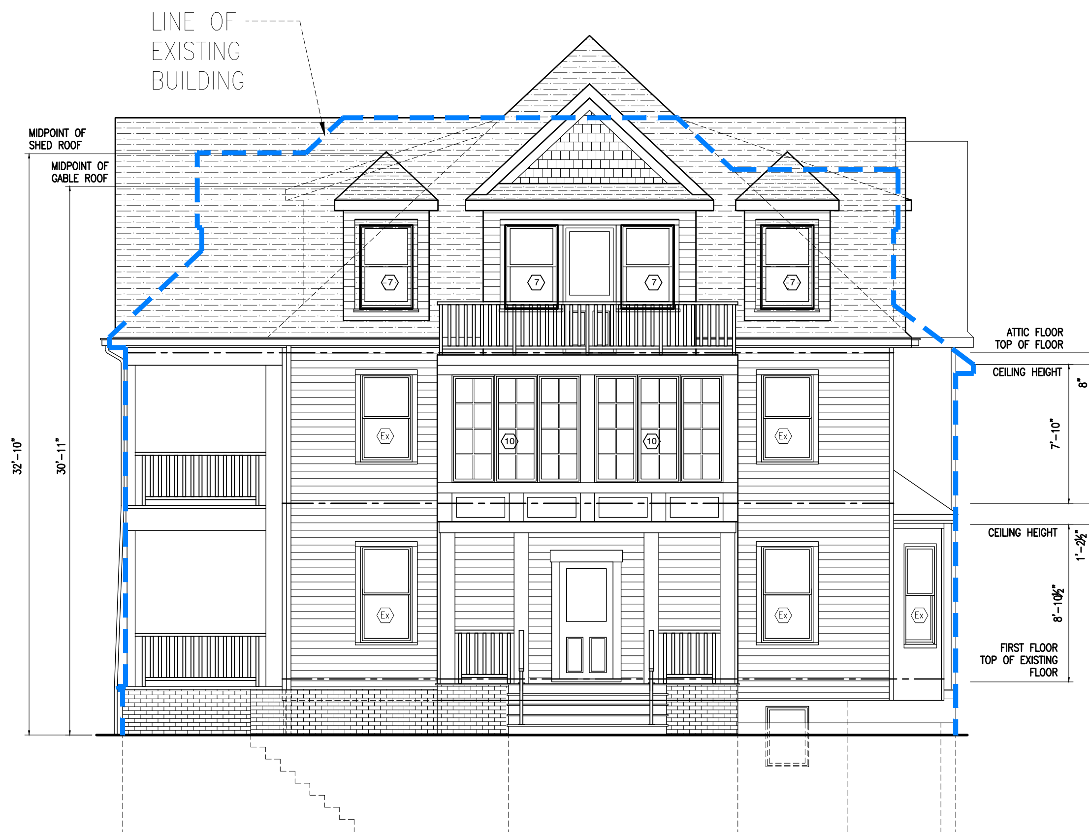
PROPOSED EAST ELEVATION ( BROADWAY ) SCALE : 3/16" = 1'-0" GRAPHIC SCALE IN FEET 0 4 8 16 32
