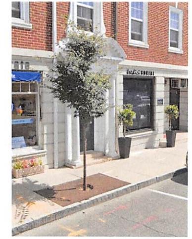
PHOTO: NEW TREE PIT WITH POROUS ASPHALT IN BRONXVILLE
