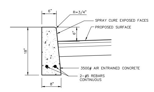
EXPANSION JOINTS TO BE INSTALLED EVERY 10 FEET. **CONCRETE CURB**
