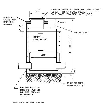
NOTE: CONC. TO TEST 4000 PSI AT TIME OF DELIVERY. RISER SECTIONS IDENTICAL TO STANDARD PRECAST CONC. MANHOLE.
