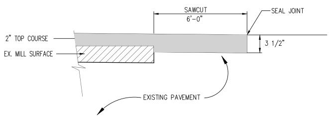
TACK COAT VERTICAL AND HORIZONTAL SURFACES TO RECEIVE OVERLAY KEYWAY-SAWCUT
