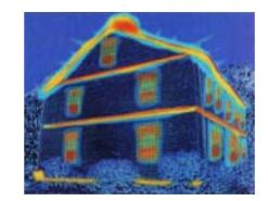
The orange and yellow stripes in the scan show indoor heated air being lost to the outdoors at typical locations where caulk and insulation should be installed.
