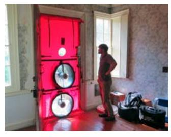
Plugging air leaks in existing buildings is key to reducing energy costs and minimizing CO2 emissions. Tools like blower doors (above) and thermal scans (below) measure air leakage and target repair efforts.
