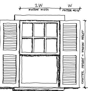
Shutters must be proportioned and positioned properly, as above, to match the window; and ideally the shutters should operate.
